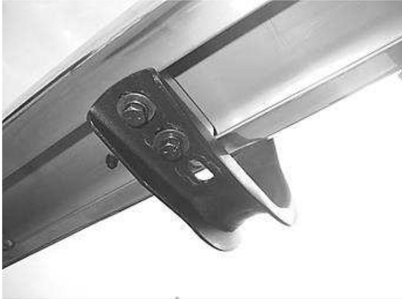
6. Repeat steps to install the passenger side brackets and side step. Remember to check and re-tighten the nuts and bolts every six months.
