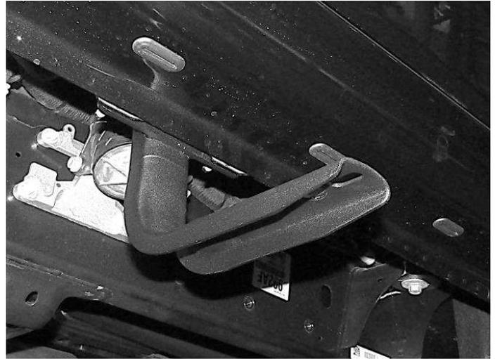
3. Locate the (3) threaded studs on the inner rocker panel at the center and rear of the cab and repeat step 2 to install two of the brackets using the supplied hardware. Note: The front mounting location is shown in Figure 3. The center and rear mounting locations are similar.
