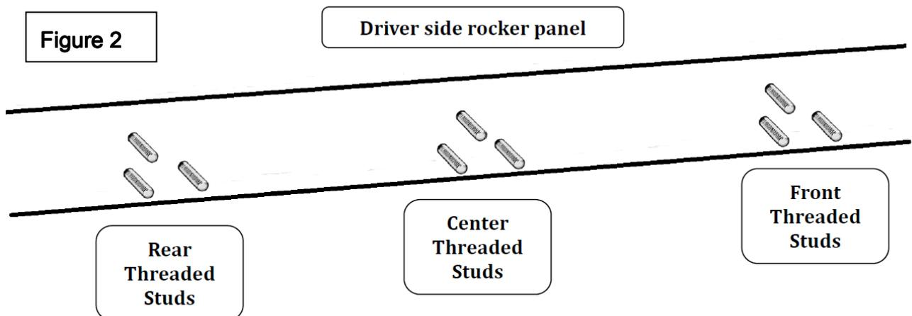
2. At the front mounting location, Install one of the brackets by positioning the bracket over the studs and secure to the rocker panel using (3) 5/16" flat washers, (3) 5/16" lock washers and (3) M8 hex nuts. Leave the nuts loose for final adjustment, (FIGURE 3). Note: The lower studs on the rocker panel may have excessive paint covering the threads. When installing the M8 hex nuts, it may be necessary to start then back off the nuts to gradually clear the paint build up.
